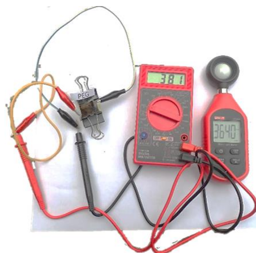
Figure 3. DSSC current and voltage measurement
