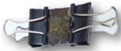
Figure 2. Construction of the solar cell electrode
